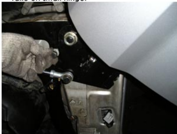
5. 맞볼트로 장착합니다. Attach the hinges to the frame using three bolts, and the car door using 4 bolts.
